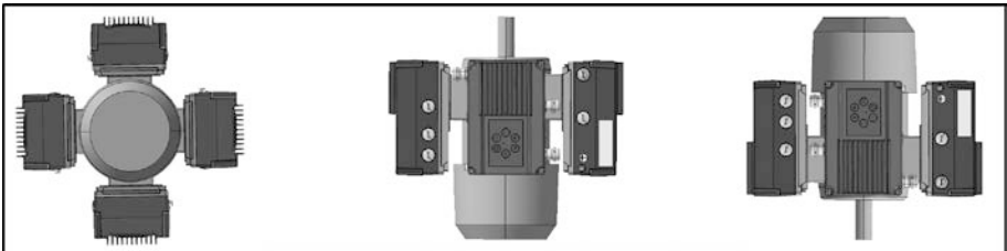
Fig.: 9 Motor installation location/permittted alignments
